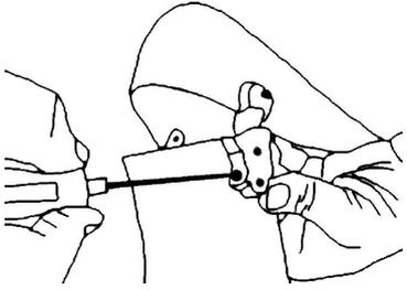
11. Install Tamarack Variable Assist Joints™ with the anchoring screws.
