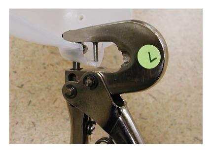
Attention: The Tamarack Hand Punch was designed to punch through polypropylene material no greater than 3/16" (5mm) thick. Attempting to punch harder or thicker materials may result in damage to the device or tool.
