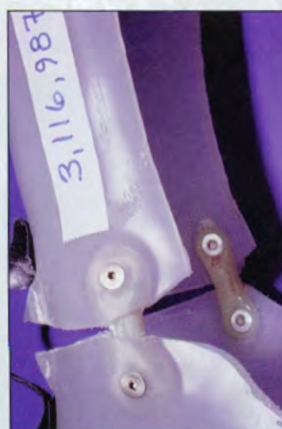
Tamarack Flexure Joints™ installed in test AFO. The AFO and joints have survived 3,116,987 cycles on the durability tester.
