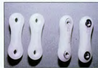
Comparing two new Tamarack Flexure Joints on the left with two joints which have served 2,229,757 cycles (no apparent damage).
