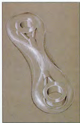
Artist's sketch of a free motion type Tamarack Flexure Joint™ showing the internal tension load-bearing element.
